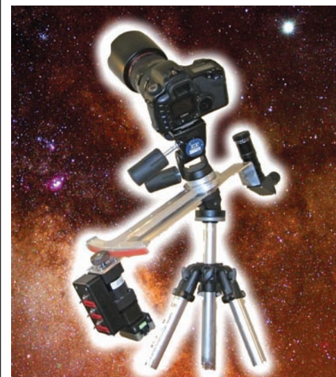
Designed to be attached to a tripod and camera, the Star-Cam Tracker allows a standard 35 mm camera to take long-exposure wide-field images of stars.
